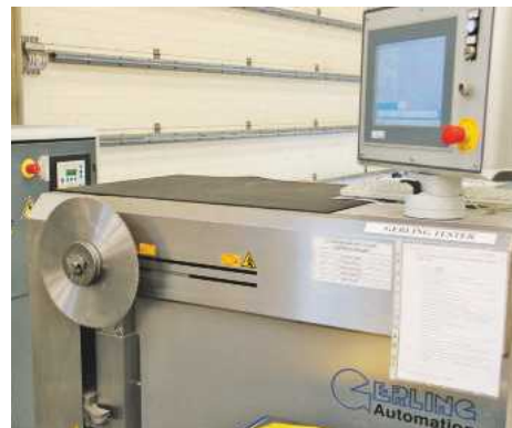
Blades go onto this machine to check them for true after tensioning
